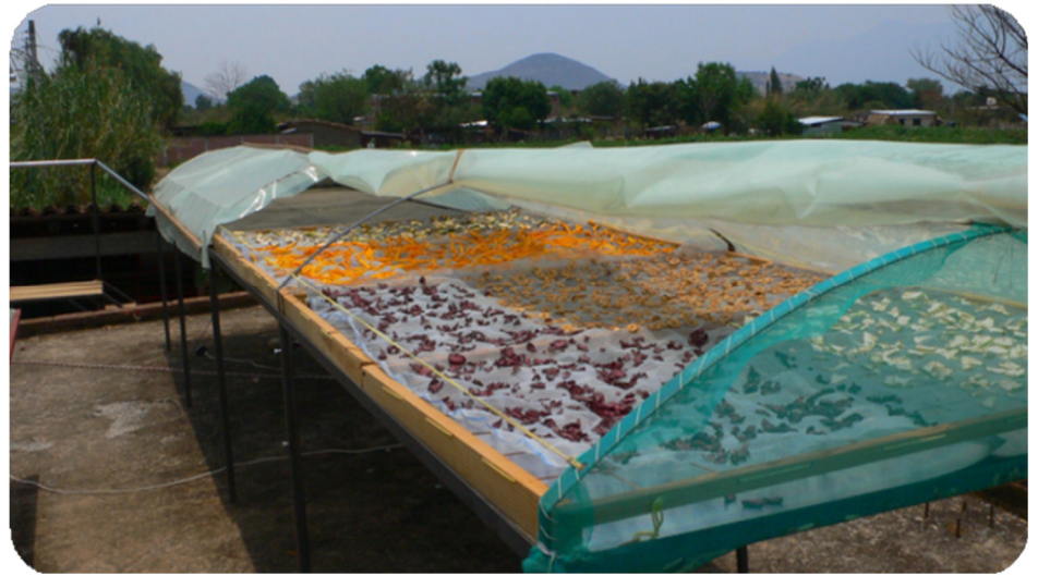
'Tunnel type' solar dryer on a rooftop in Mexico (opened to show the fruit inside)
