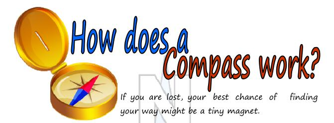
A magnet is what makes a compass point North. The small magnetic pin in a compass is suspended so that it can spin freely inside its casing and respond to our planet's magnetism.
