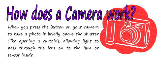
In daylight situations the shutter may be open for just 1/200 of a second, in darker situations the shutter needs to stay open for longer, perhaps a few seconds, or even much longer in dark, night-time environments.
